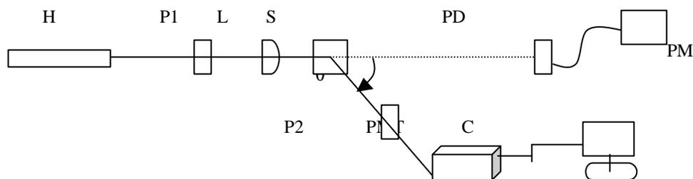
Fig. 1 Schematic diagram of the Light Scattering set up
