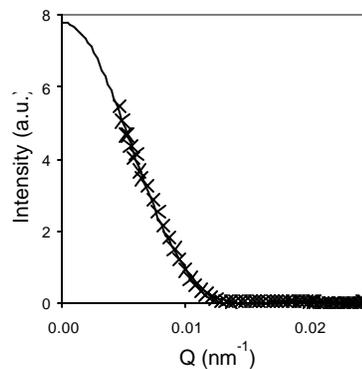
**Fig. 2** Photograph of Light Scattering Set up**Fig. 3** SLS data and fit for 300 nm Polystyrene latex
