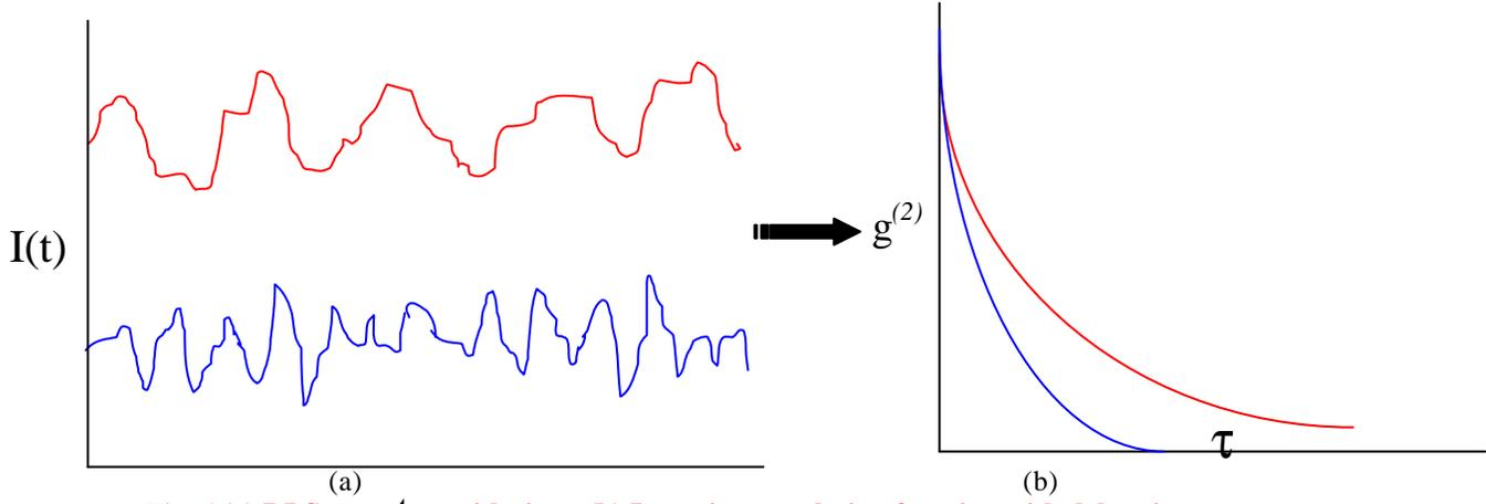
**Fig. 4 (a) DLS spectrum with time; (b) Intensity correlation function with delay time**
