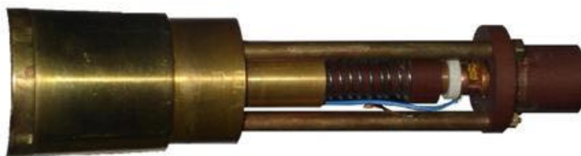
fabricated sample-cell for permittivity measurements at cryogenic temperatures
