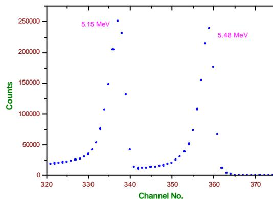
Energy spectrum of SSB detector made from irradiated silicon wafer
