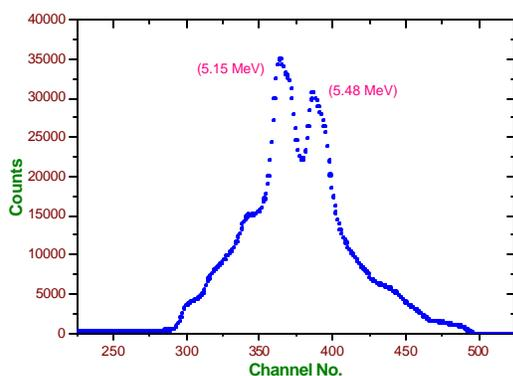
Energy spectrum of SSB detector made from as-irradiated wafer using an alpha source
