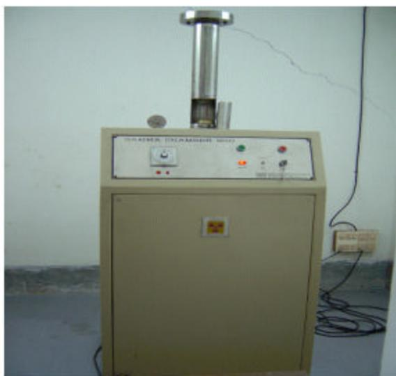
Gamma Irradiation Chamber commissioned at UGC-DAE CSR, Kolkata Centre is the GC 900 model, procured from BRIT, Mumbai. Both solid and liquid samples can be irradiated. A liquid sample holder for 12 samples in test tubes of 10 mm diameter is fabricated. Following are some other details of the Radiation Facility :
