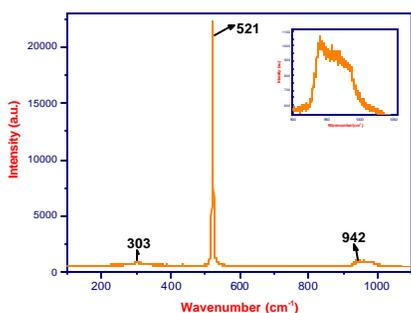
Fig. 1: Raman spectrum of Si(111) wafer.
