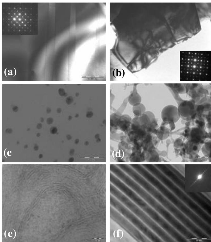
Fig. (a) Microstructure and diffraction from twined domains in  $\text{Sr}_{0.7}\text{Ca}_{0.3}\text{TiO}_3$
