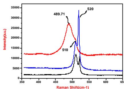
Fig.2: Raman spectrum of porous Si nano-particles.
