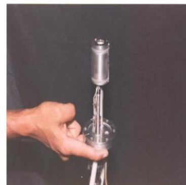
A versatile Knudsen type effusion cell has been fabricated for growing nanostructures and epitaxial layers of metals and semiconductors. The cell provides excellent vacuum compatibility ( $10^{-10}$  mbar range during operation), efficient water cooling, uniform heating, and moderate input power consumption (100 W at 1000 °C). Rev. Sci. Instrum. 75, 4467, 2004.
