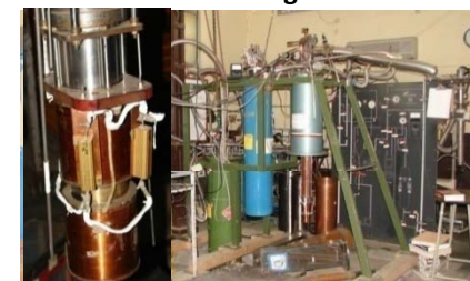
Liquid Nitrogen Plant Linit 50
